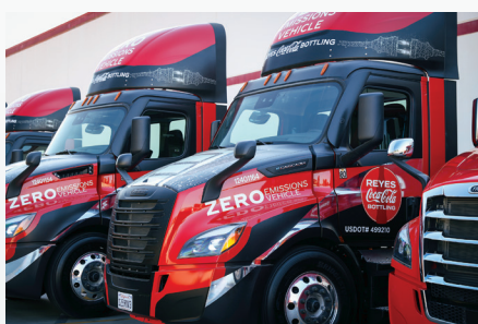
20 Battery Electric Freightliner eCascadias will rely solely on 20 Detroit eFill commercial charging stations that have been installed at the Reyes Coca-Cola Bottling Downey facility.
